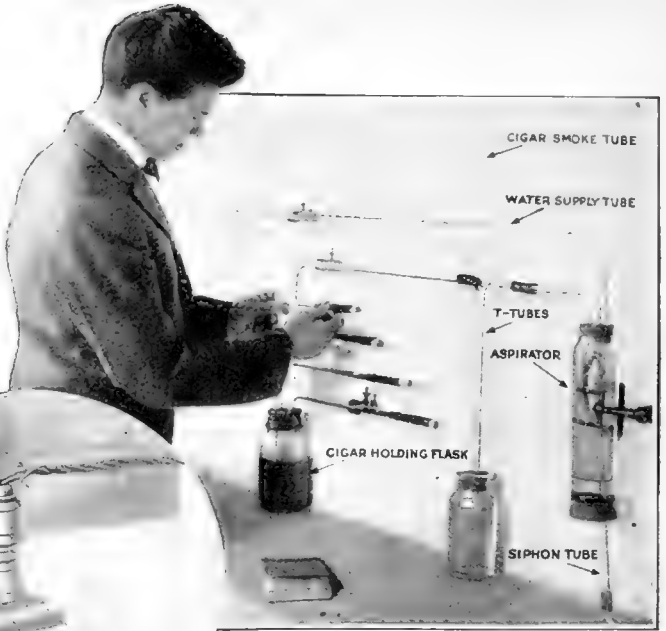
Above, the aspirator and siphon apparatus for testing tobacco leaf. It smokes four cigars in thirty minutes. At left, the blower outfit which is operated by electricity. The smoke is coming from the exhaust outlet
